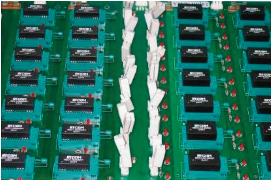
Fig. 7.2: DC/DC converters being tested in a burn-in chamber ( T_{AMB} = 40^{\circ}\text{C} )
